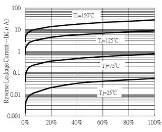
Reverse Leakage Current vs Reverse Voltage
